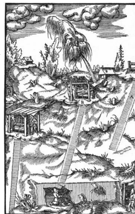
THREE DRAFTS OF WHICH A DOES NOT YET REACH THE FUNNEL; B REACHES THE FUNNEL; IN THE THIRD, C, THE FUNNEL HAS NOT YET BEEN SHOWN. 20-300000
